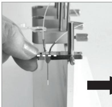
3. Insert the probe into the clip gap so that the upper level of the clip is linear to the upper level of the probe head.
