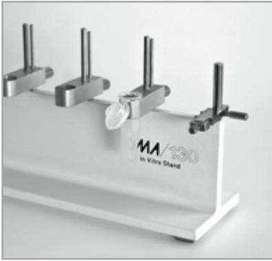
1. Fix a probe clip to the vertical pin at one end of the stand.
