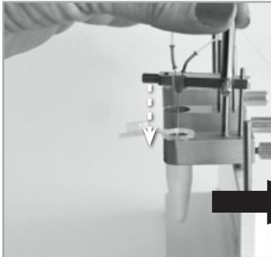
5. Move the probe clip with the probe and attach it to the vial holder. Secure it to the stand with the lock screw. You can now wash, test or store the probe.
