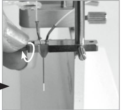
4. Turn the screw on the clip clockwise to tighten the probe to the clip. The shaft of the probe will now be vertical.
