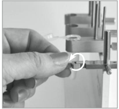
2. Open the probe clip by turning the lock screw counterclockwise.
