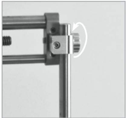
8. Connect the assembly to the frame with the screw on the stereotaxic adapter.
