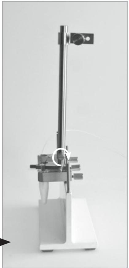
6. Attach the connecting rod and stereotaxic adapter to the clip. Lock them together with the screw on the connector.
