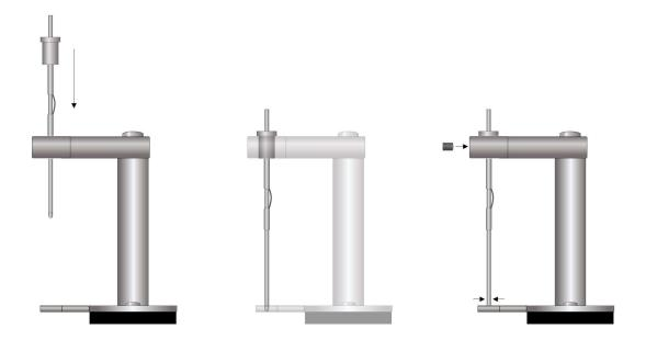
Secure the cannula to the tower arm with the screw. Make sure that the cannula is centered in the lower hole by adjusting it using fingers when tightening the screw.
