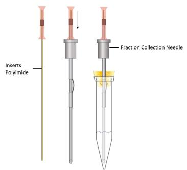
If a risk of carry-over effects between experiments is suspected, the insert can be easily disposed of. The Insert lower the internal dead volume. Checking the actual dead volume see description below. There is a risk of
